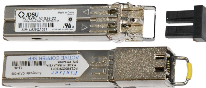
Figure 18 Optical or copper SFP transceiver module
