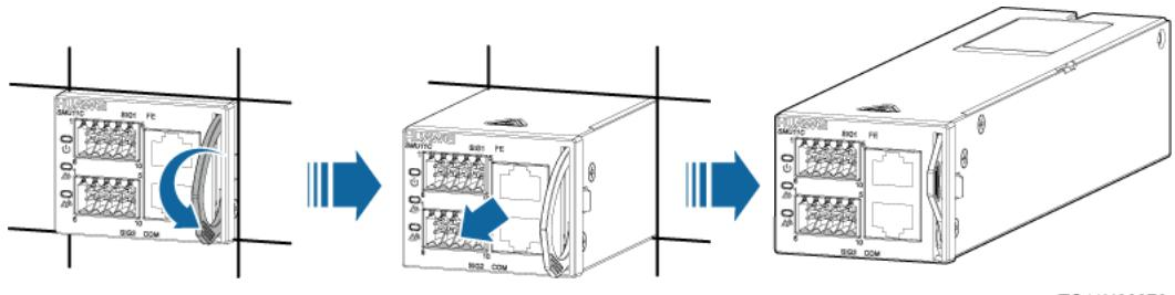
**Step 4** Insert the new monitoring module into the corresponding slot and push it into the slot along the guide rails.
