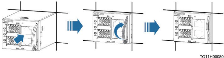
**Step 6** Connect the signal cable terminals and COM communications cables to the panel of the new monitoring module based on the recorded information.
