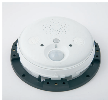
Attach the ExtIO to mounting ring
