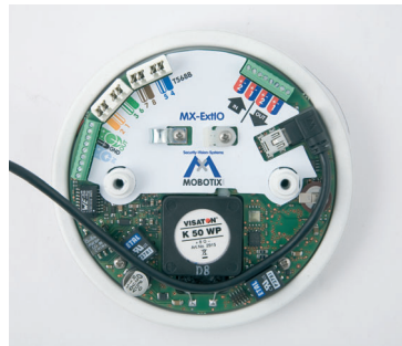
Insert USB plug Properly guide the cable
