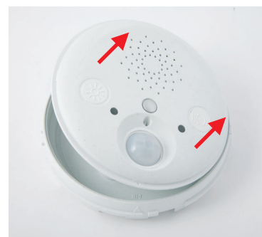
Remove the back of the housing
