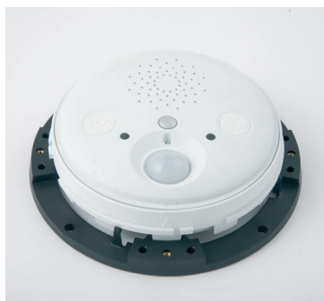
Attach the ExtIO to mounting ring
