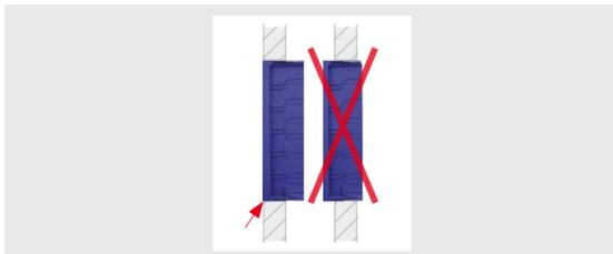
Set the protective cardboard cover (included with the delivered parts) into the housing before pushing it into the cavity. This prevents cement from entering the interior of the housing. After you have installed the housing
