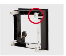
2. To facilitate the installation, there are notches for the clamping brackets on three corners of the FlatMount Frame. After you have attached the long clamping brackets to the FlatMount Frame, turn three of the clamping brackets so that they fit into the notches. Turn the fourth clamping bracket (on the corner without notch) downwards.
