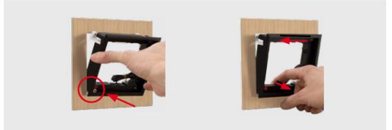
**Caution:** In situations, in which a theft protection is not necessary, e.g., indoor installations, **do not** activate the theft protection (the red knob remains in the "open lock" position). If you twist the knob by mistake, you have to be able to attach a battery (9 V DC) to the theft protection wires! Otherwise, you will not be able to remove the module from the frame any more.
