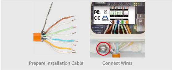
**Note:** To release a wire, unlock the terminal by pressing with the screwdriver (included with delivery) into the opening above the wire. Then pull out the wire.
