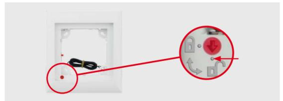
**Caution:** In situations, in which a theft protection is not necessary, e.g., indoor installations, **do not** activate the theft protection (the red knob remains in the "open lock" position). If you twist the knob by mistake, you have to be able to attach a battery (9 V DC) to the theft protection wires! Otherwise, you will not be able to remove the module from the frame any more.
