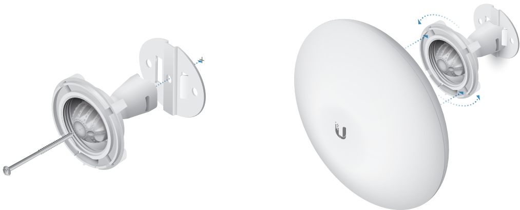
Installation Using the NanoBeam Wall Mount Kit
