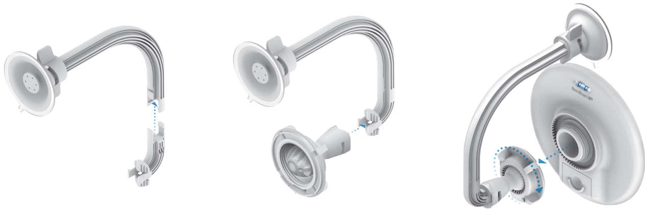
Installation Using the NanoBeam Window Mount
